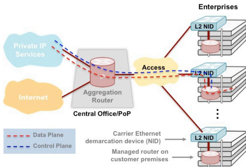
A better approach is to deploy only a simpler OpenFlow-enabled NID at the customer site, obviating the need to install and manage a separate router. Similarly, in the central office the expensive aggregation router can be replaced by a more cost-effective Layer 2+ OpenFlow-enabled switch (see Figure 6).
