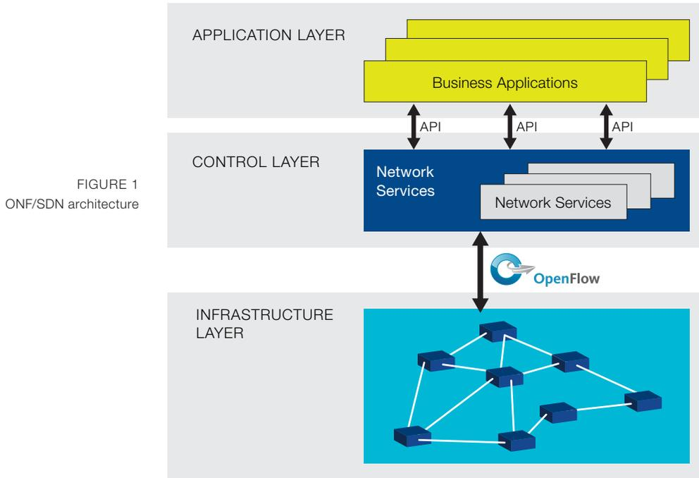
The ONF/SDN architecture consists of three distinct layers that are accessible through open APIs:
