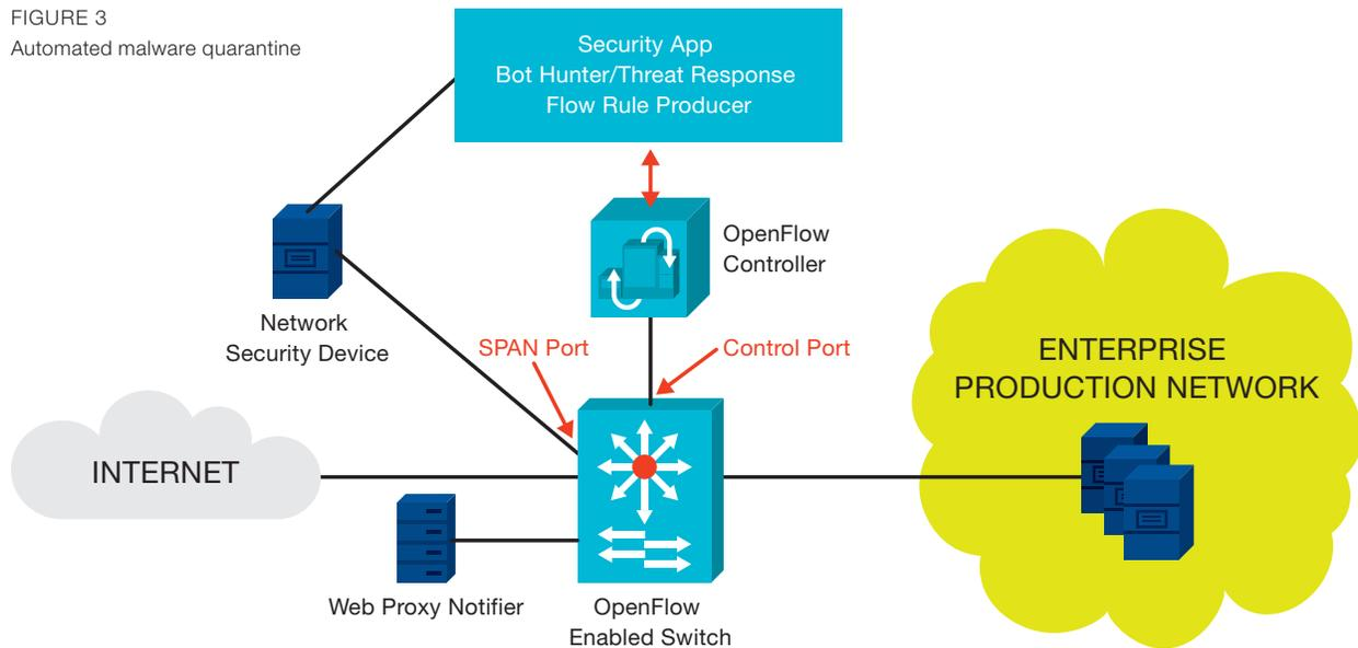
OpenFlow-based SDN enables a more flexible approach for AMQ, as illustrated in Figure 3. AMQ functionality is centralized in the SDN controller, where it provides efficient security processing. Only suspicious flows will be isolated and monitored.
