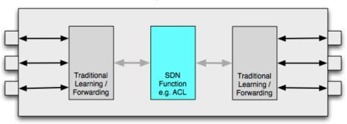
Figure 12: SDN Controlled Function in Traditionally Controlled Datapath
