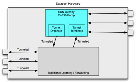
Figure 11: Overlay On/Off-Ramp Gateway
