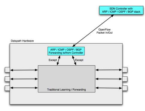
Figure 14: Traditional Control Plane On SDN Controller
