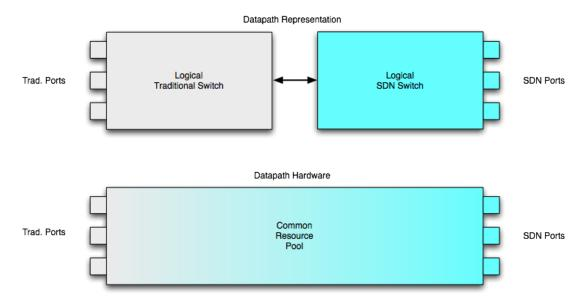
Figure 10: Port Oriented Hybrid with Common Resource Pool
