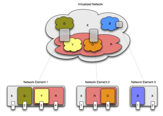
Figure 7: Virtualized Network and Virtualized Network Elements
