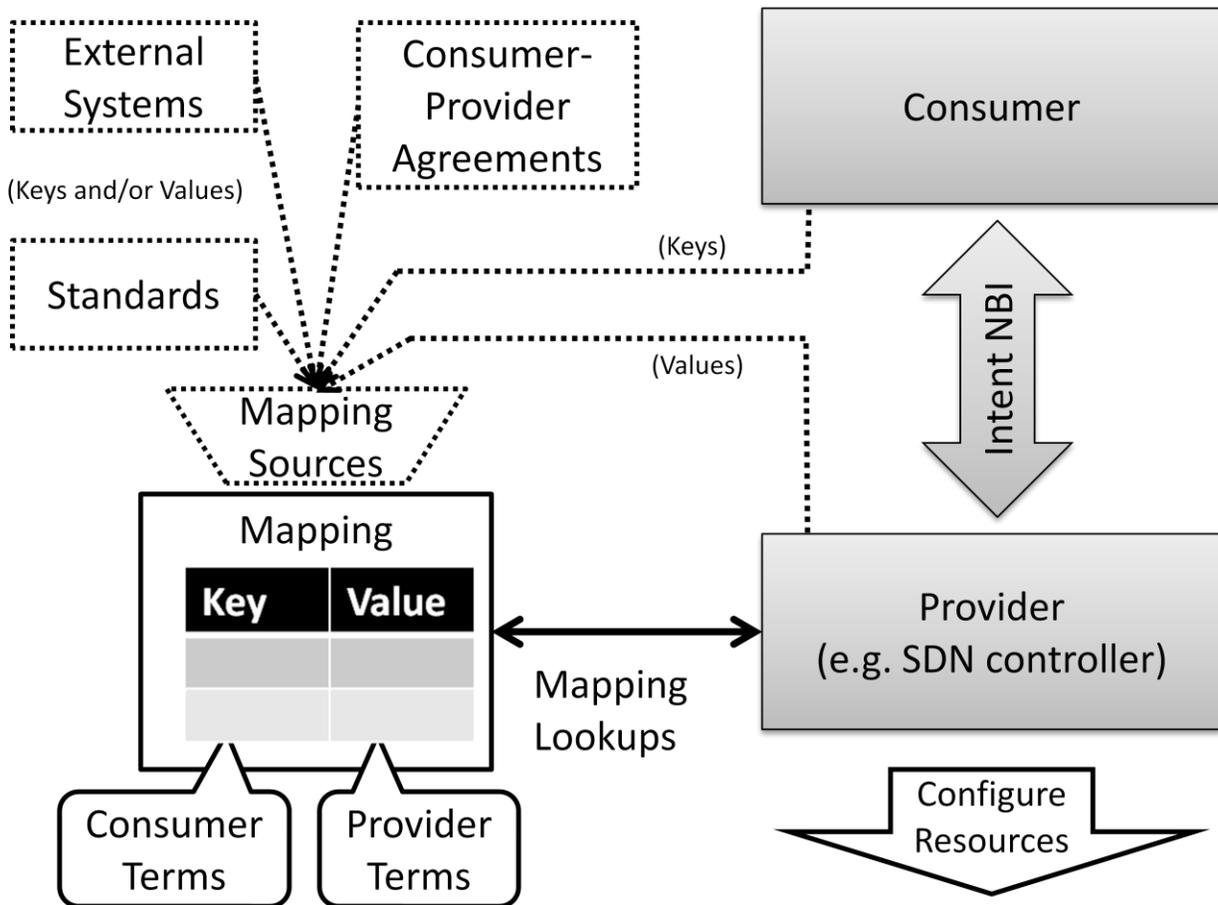
**Figure 4 Architectural representation of Intent NBI, mapping and potential sources of mapping contents and/or their dynamic updates. The illustration of mappings as standing outside of provider systems is not prescriptive.**
