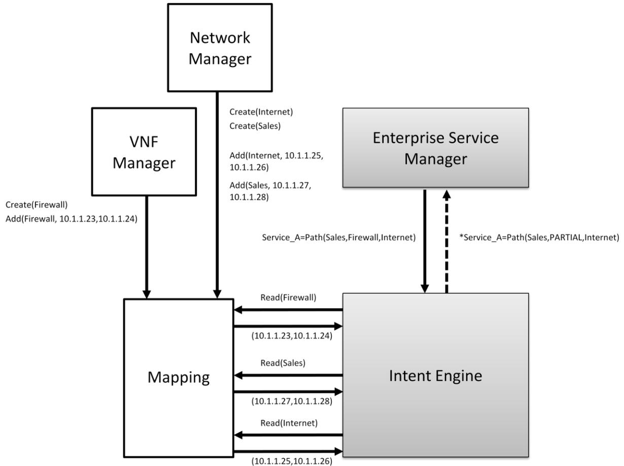
**Figure 6 An example of Intent NBI system operation for a simple service function chaining use case. The specific Intent NBI and mapping API syntax/expressions are hypothetical examples.**
