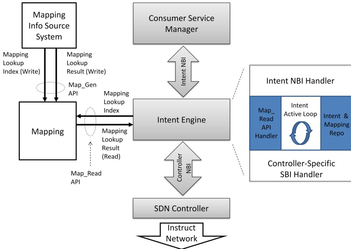
**Figure 5 Schematic representation of "engine" implementation of Intent NBI (such implementation is not prescriptive). The illustration of mappings as standing outside of the Intent engine and provider systems is not prescriptive.**
