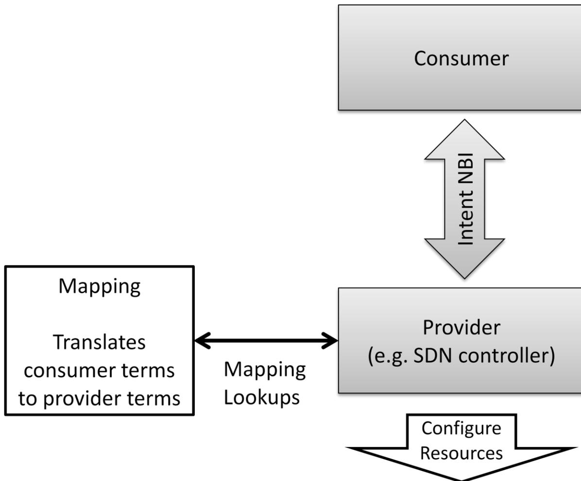
**Figure 1 Architectural representation of Intent NBI and mapping. This representation is nominal and not prescriptive (e.g., implementations may place mappings within provider system architectures).**
