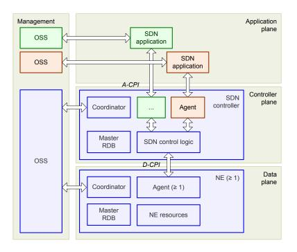
Figure 1: OpenFlow SDN reference model, from [1]
