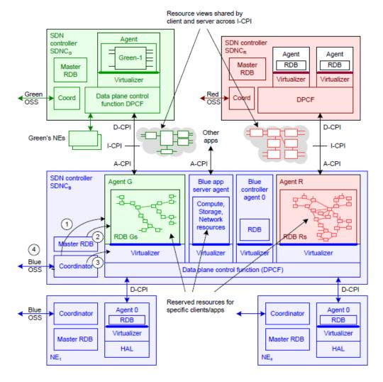
Figure 3: Virtual network, single-level control hierarchy, from [1]
