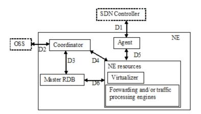
Figure 4: Data Flow Diagram (DFD) for an SDN NE
