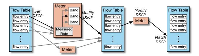
Figure 5: Meters and Hierarchical DSCP metering.
