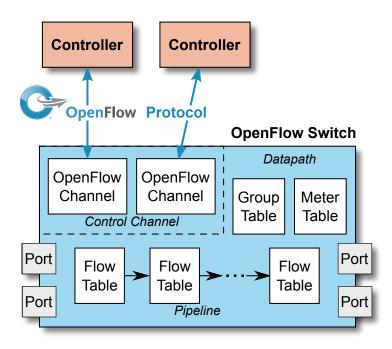
Figure 1: Main components of an OpenFlow switch.
