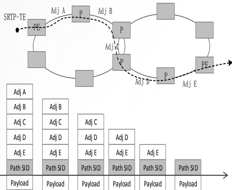
**Path SID Distributed:** the destination nodes distribute the Path SID to source node
