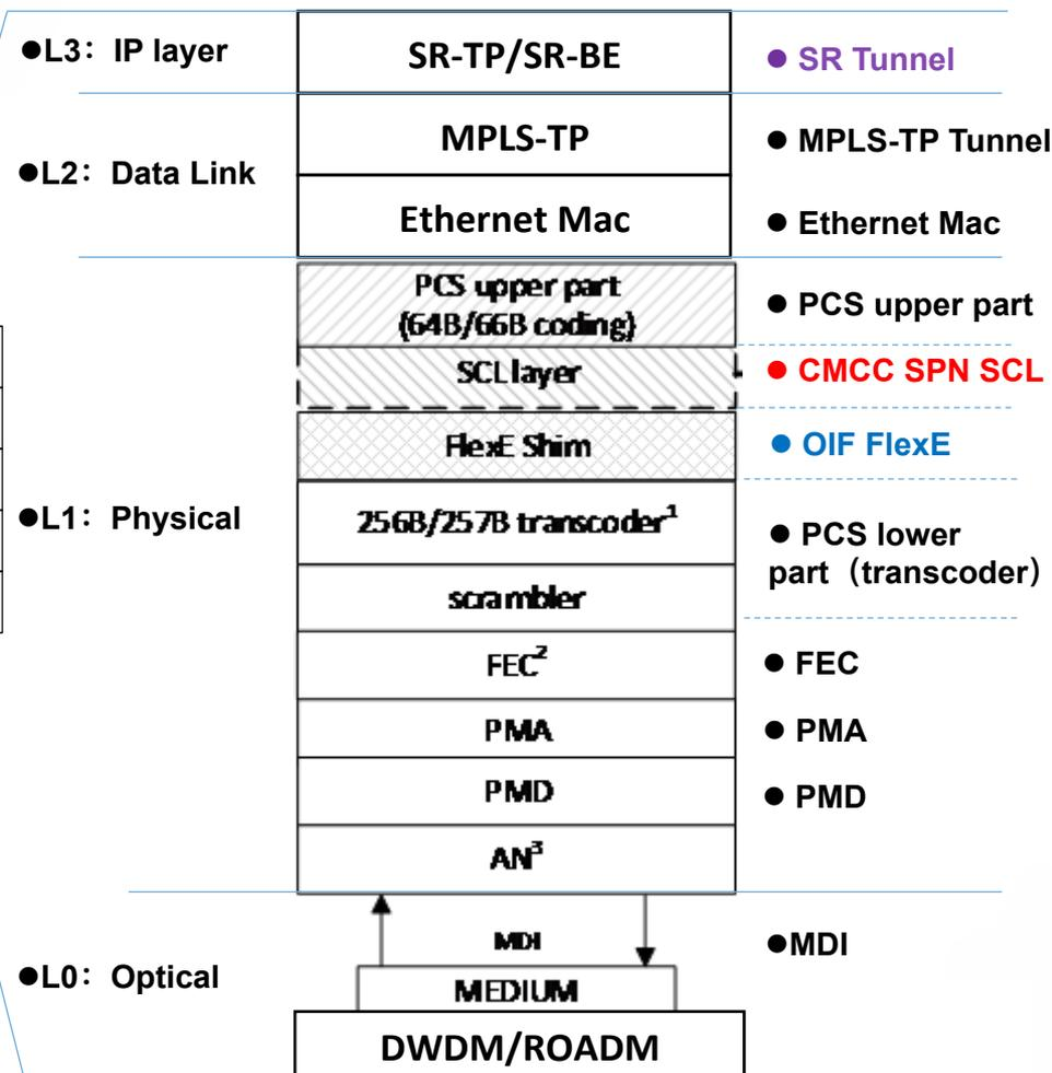
SPN innovatively introduces SPN channel layer, integrates TDM and packet switching, and integrates L0 layer to L3 layer into a whole.
