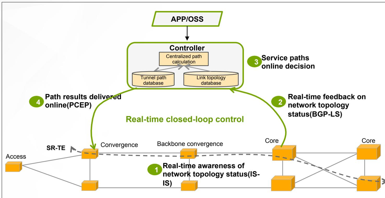
With the combination of IS-IS、BGP-LS and PCEP protocols, SPN realizes real-time closed-loop control of service paths.
