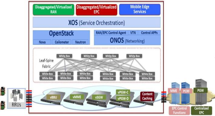
Architecture: It is based on the CORD components or OpenStack as VIM, ONOS as controller SDN and XOS as local orchestrator of the individual components. Dedicated infrastructure created by Radisys with VRAN and vEPC
