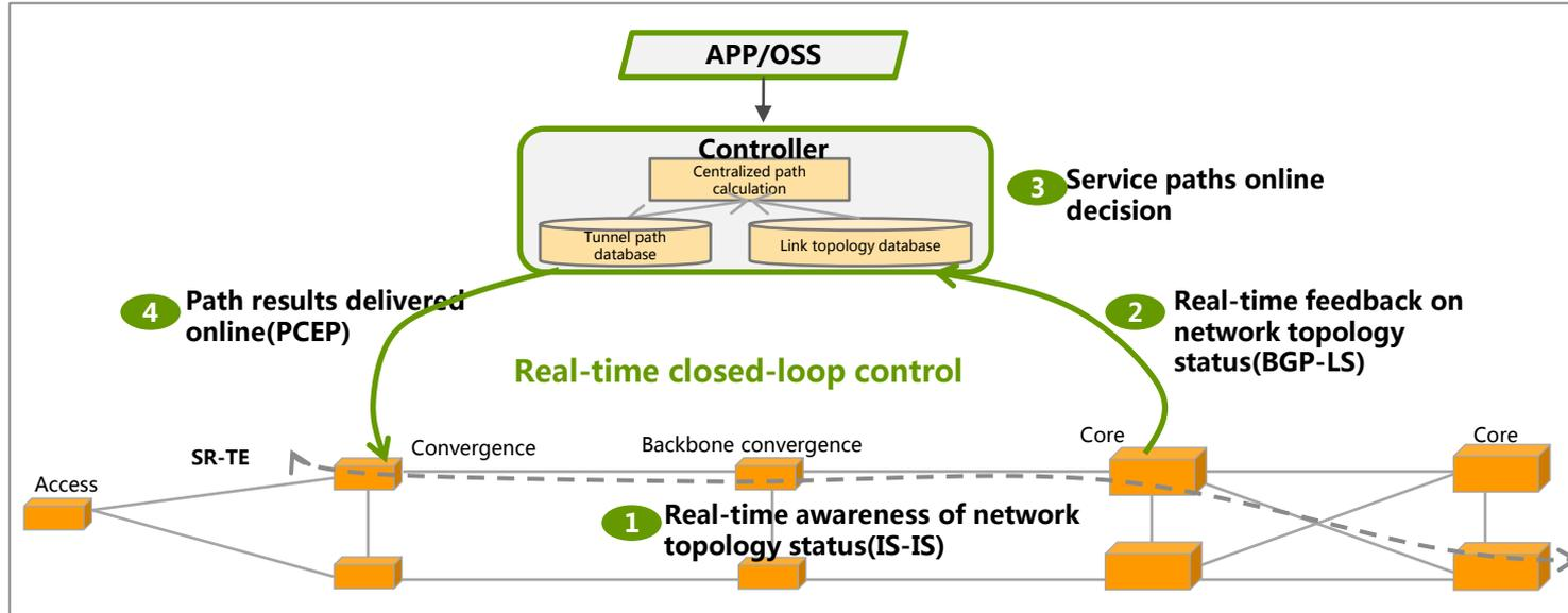
With the combination of IS-IS, BGP-LS and PCEP protocols, SPN realizes real-time closed-loop control of service paths.
