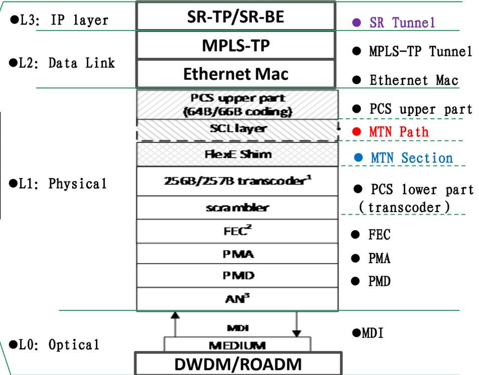
SPN innovatively introduces SPN channel layer, integrates TDM and packet switching, and integrates L0 layer to L3 layer into an organic whole.
