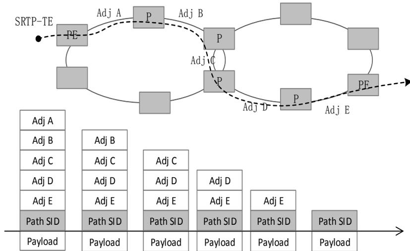
**Path SID Distributed** : the destination nodes distribute the Path SID to source node
