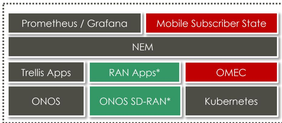
SD-RAN controller based on ONOS applications which is hardened for deployment
