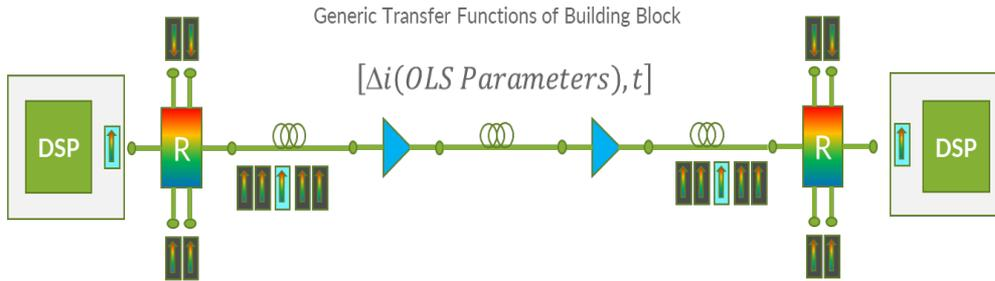
$$\overline{O}(BER(FEC), P_{out}, OSNR, DSP, \dots) = [\Delta(OLS\ Parameters), t] \overline{I}(BER(FEC), P_{in}, OSNR, DSP \dots)$$
