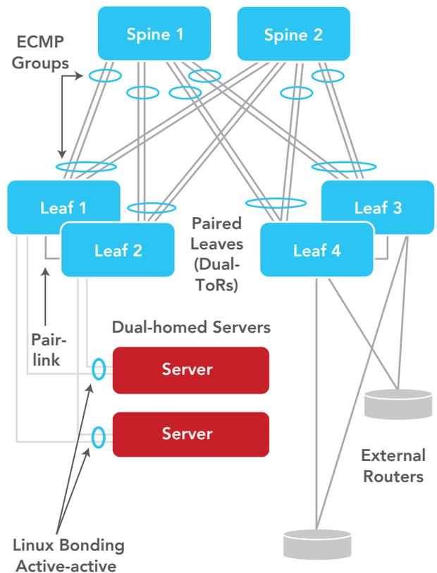
**Horizontal Scaling & Redundancy.** Trellis allows horizontal scaling of the fabric. Operators can start off with simply a single switch or two (for redundancy). As needs grow, they can add more spines and more leaves to their infrastructure seamlessly. This feature supports both scale and redundancy built into both spine and leaf layers as well as the control-plane which is based on a high-performance, scalable and resilient ONOS cluster.
