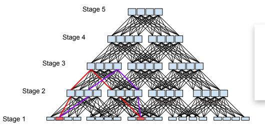
Large virtual switch built out of small commodity switches
