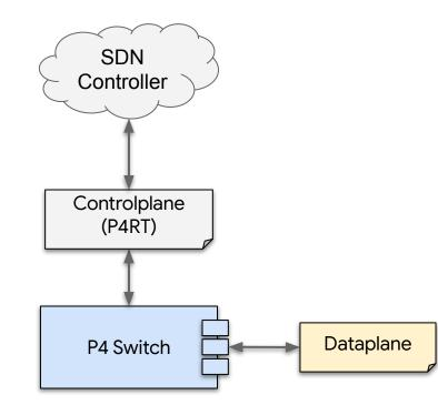
Dataplane testing requires packets that trigger all switch behaviors
