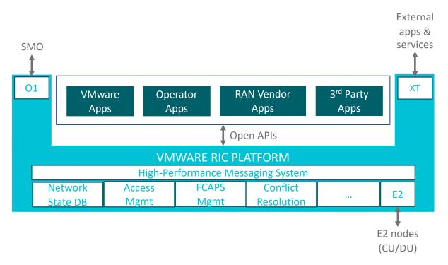
**XT (External) Interface** is VMware feature to enable **edge intelligence** beyond RAN (i.e., to provide capabilities for RAN insights & optimizations to external services and applications)
