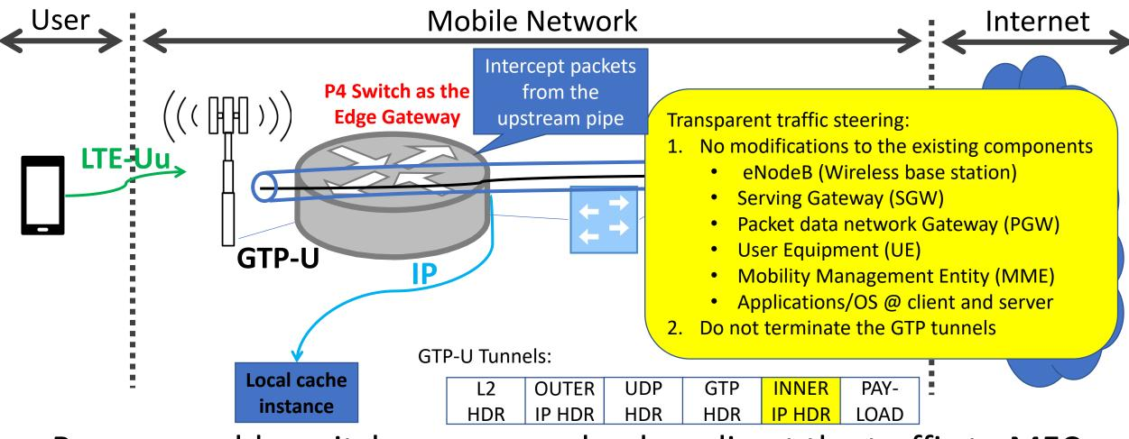
Programmable switches can seamlessly redirect the traffic to MEC
