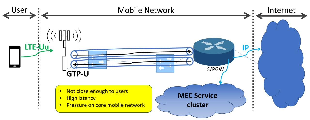
Intermediate devices cannot terminate GTP tunnels; MEC services have been deployed at PGW or IPX that connects PGW to the Internet
