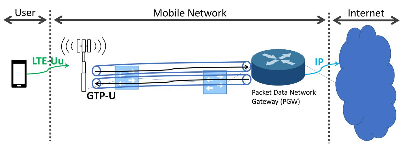
Mobile networks use GPRS Tunneling Protocol to connect to the Internet
