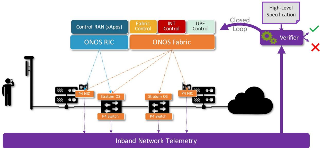
Figure 4: Pronto supporting verifiable closed-loop control
