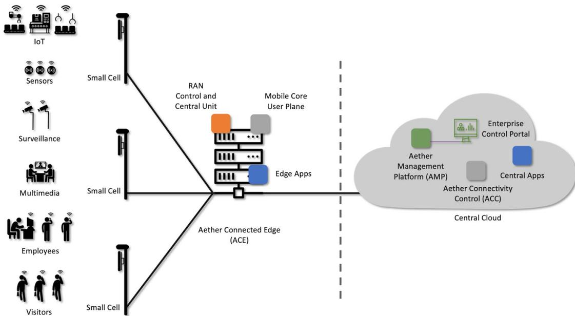
Figure 2: Aether providing Enterprise-5G/LTE-Edge-Cloud-as-a-Service
