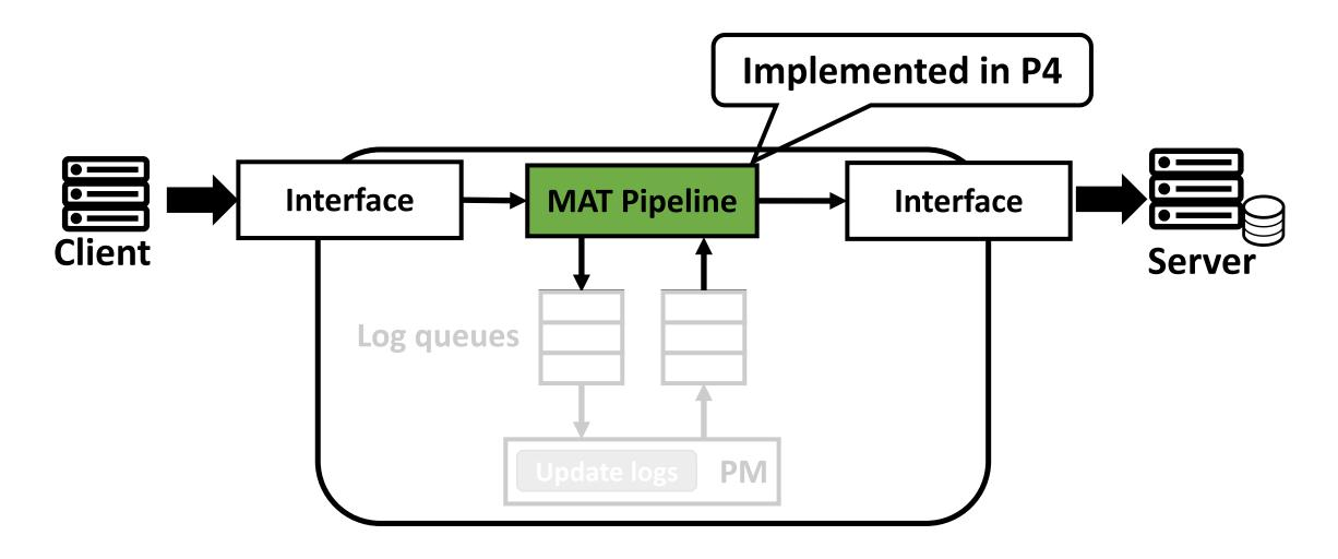
PMNet MAT Pipeline is compatible with P4-supported network devices
