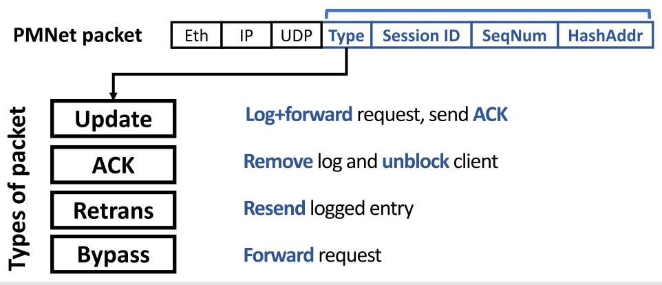
PMNet performs different operation based on packet type
