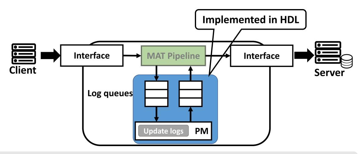
Request queue and memory controller are implemented in HDL due to lack of persistent storage support
