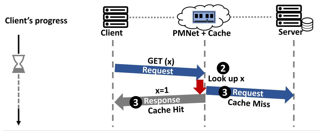
PMNet exploits logged entry and recovery mechanism to respond read requests.
