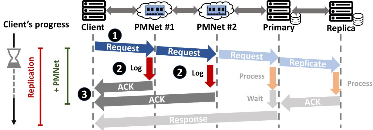
PMNet exploits **persistent logging** to move replication off the critical path
