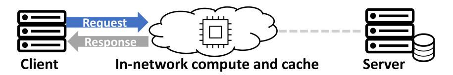
**In-network compute** [Brainwave NPU ISCA'18, iSwitch ISCA'19, E3 ATC'19, iPipe SIGCOMM'19]
