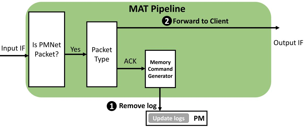
PMNet ACK **removes** the logged entry
