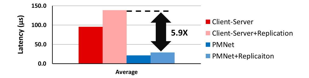
PMNet reduces replication latency while offering the same level of fault tolerance.
