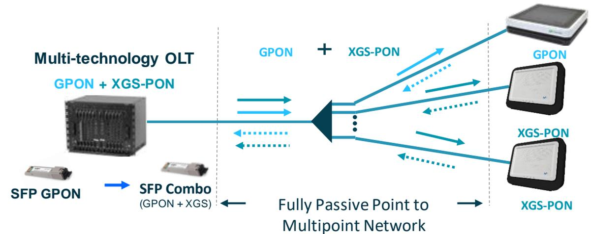
Multi-PON OLTs can work with only GPON, only XGS-PON and simultaneously GPON & XGS-PON, allowing the simplest migration path from GPON to 10G, port by port.
