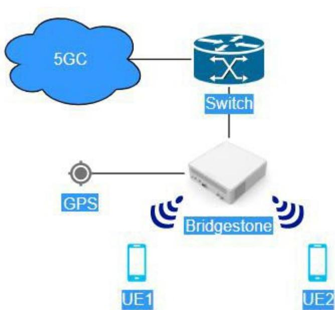
Using this topology need to enable WAN progress, GPS\_SYNC progress and NR progress.
