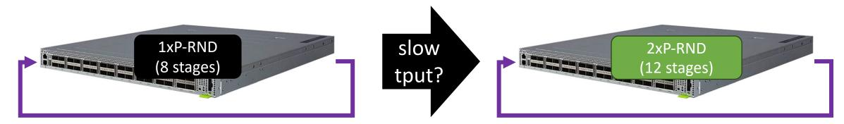
**packet recirculation**: add *special* metadata header to the packet to store the current P-RND number and relevant states. **double the P-RNDs**: mutually exclusive operations can be parallelized while sharing the pipeline stages
